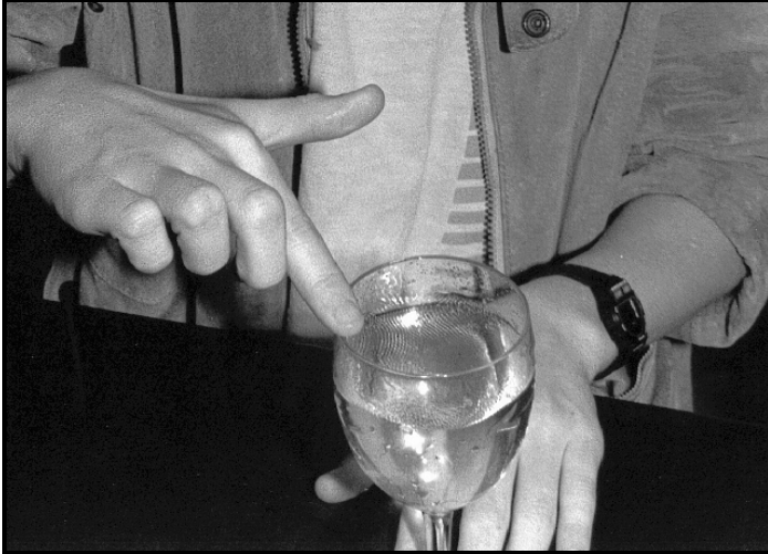
Figure 8.1: If a wet finger is pushed around the edge of a wine glass filled with water, vibrations are set up, which cause a high-pitched, pleasant sound. Notice the waves that are generated in the water by the vibrations of the glass.
